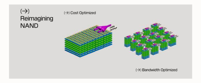
To help address this critical gap, Sandisk developed a revolutionary new memory technology: High Bandwidth Flash (HBF $^{\text{TM}}$ ). HBF is built from the ground up for AI inferencing. With up to 16x the capacity of HBM4, HBF offers industry-leading capacity at similar bandwidth and similar cost.
