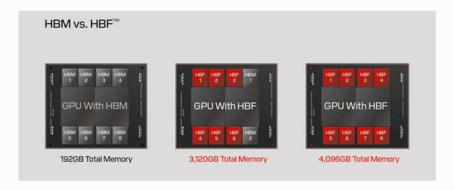
The first-generation product delivers blazing-fast read bandwidth of 1.6 TB/s and packs 256Gb per die, reaching 512GB² total capacity per 16 die stack while closely matching the physical footprint, power profile, and stack height of HBM4. HBF is purpose-built to meet the scale and intensity of next-generation Al inference workloads, offering the performance needed without compromising on capacity or efficiency.
